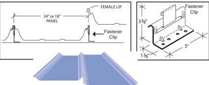
Architectural Standing Seam Roof Panels are generally narrower in width (12", 16" or 18") and have shorter high ribs that are bent at a 90-Degree angle. Architectiral Roofs have a minimum pitch of 3:12 or where hip-conditions are used (Detail at Left)
